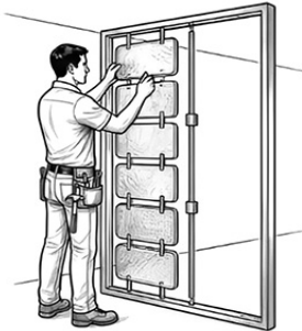
3. Slide Small Glass Panels in Place & Install Next Row
