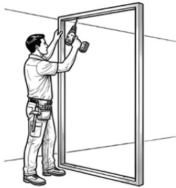
1. Secure Main Metal Frame to Floor and Ceiling
