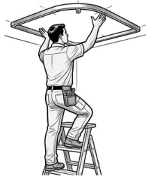
2. Secure Taped Frame to Ceiling and Check Alignment (Stick Fix)
