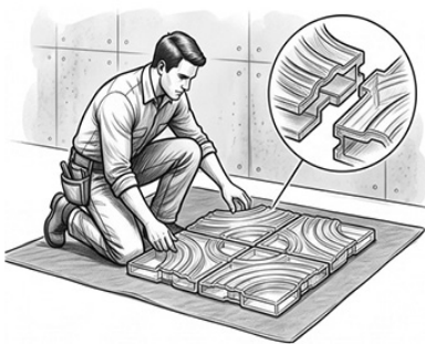
1. Lay and Interlock Glass Pieces on a Flat Protective Surface
