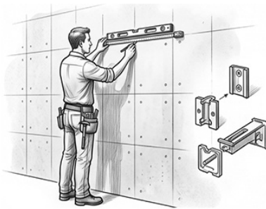
1. Mark Layout and Prepare Individual Wall Anchor Clips
